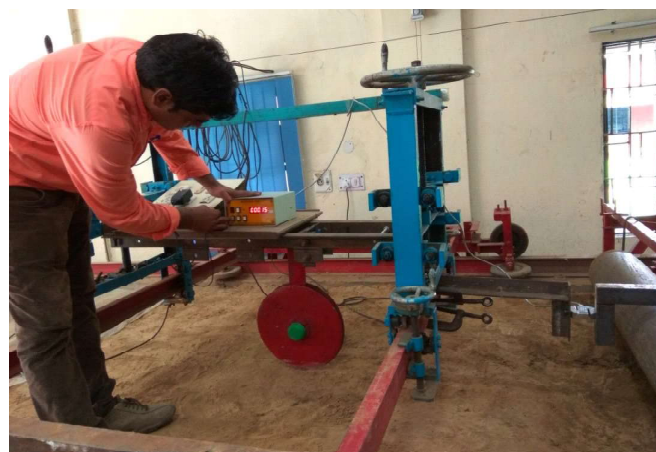
Figure 2. Experimental setup for measurement of force in Soil bin.
