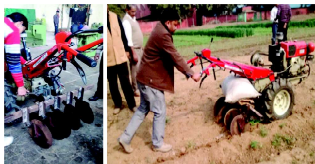
Figure 3. A small scale prototype of double disc furrow opener & its field operation.
